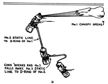
FIGURE 15.—Operation of a "daisy chain."
