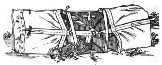
FIGURE 9.—Type A-5 aerial delivery container, showing base plate rig for dropping 81-mm mortar complete. The barrel and bipod are inside the roll.
